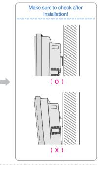
**5** Check installation and install filter and front cover on the product.
